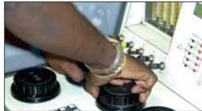
Multiple-sample pycnometers (such as Quantachrome's Pentapyc 5200e) dramatically reduce operator time.
